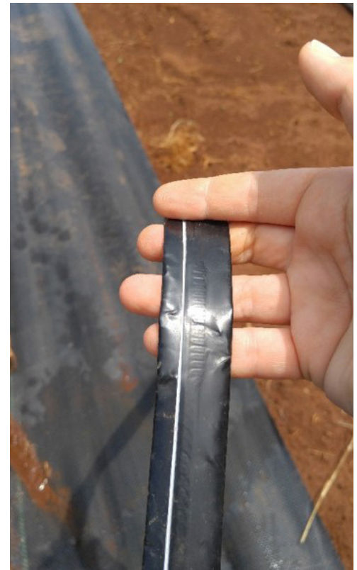
FIGURE 11. Close-up view of drip tape showing internal emitter embedded in the plastic. This tape had emitters at 12-inch spacing. (Image source: Natalie Bumgarner)
